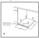
With the appliance installed adjust all four feet ensuring the machine is stable, and a clearance of approximately 5
